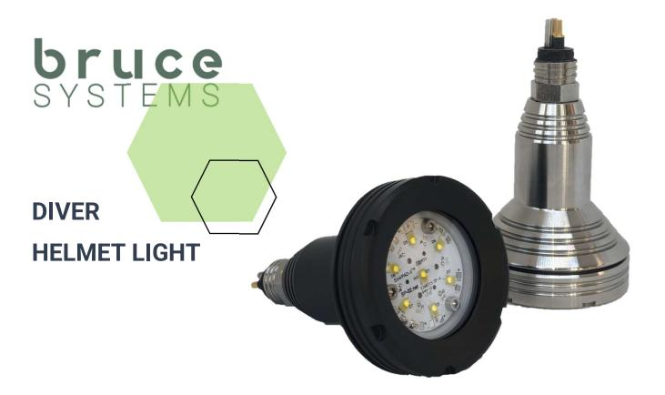
The Diver Helmet LED light has build-in electronics which automatic compensate umbilical lenghts and current. A 24 VDC power source will give optimum results, only for long cable (> 250 meters) it is recommended to use 36 VDC power source. Bruce Systems Helmet LED light is also available with a different connector and locking sleeve on request.
